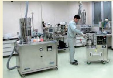
Mixing and granulation room Machines are placed in zones depending on the process they are used for
