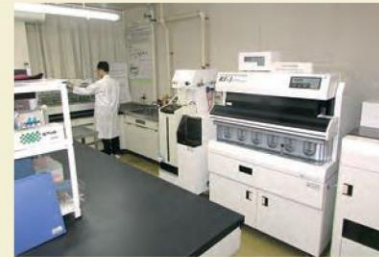
Equipment room Both manual type and automatic elution test device are placed.
